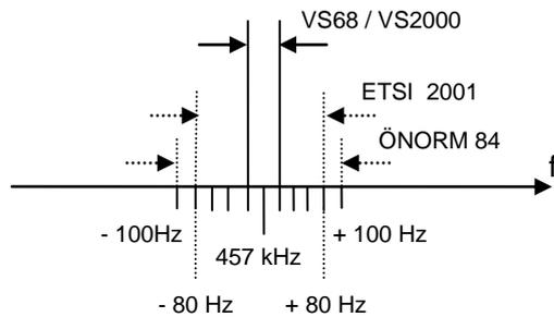
Fig. 3 Frequency tolerance VS 68 / VS 2000
