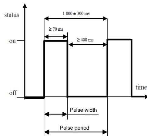
Fig. 12 ETSI A1A carrier keying specification [8]
